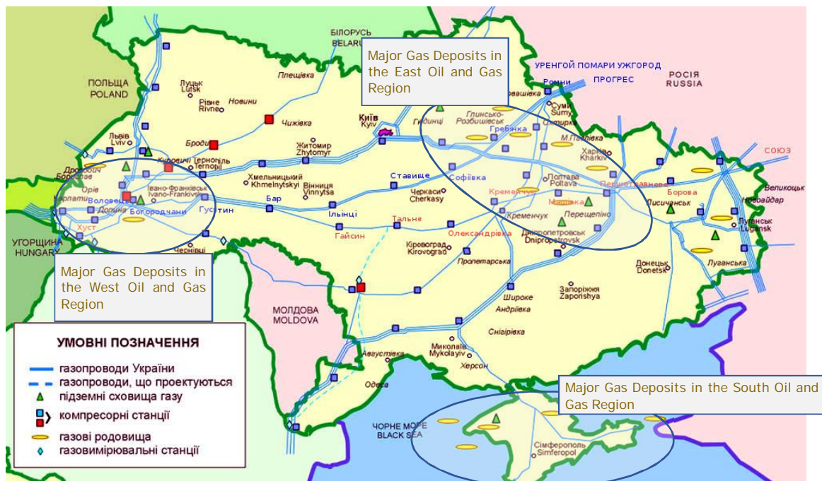
Figure 3.13 – Routes of Major Gas Trunk Lines Operated by PJSC Ukrtransgaz Relative to Core Oil and Gas Regions of Ukraine
